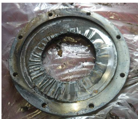
(a) 压接错位的防爆膜
